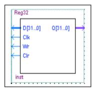
Question 2.2.1: What is the fastest clock rate that your 32-bit register can operate at correctly (remember that clock rate is not the same as worst-case propagation delay)?
