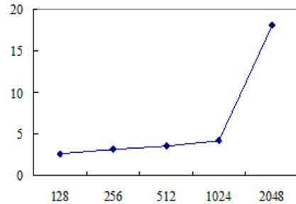
Fig. 8. Speedup ratio of matrix multiplication
