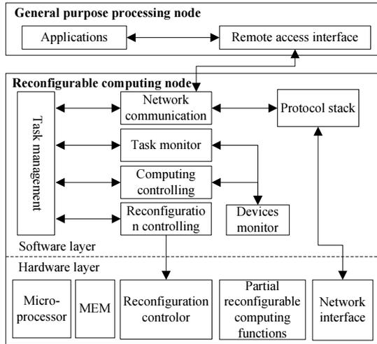
Fig. 1. System function module architecture
