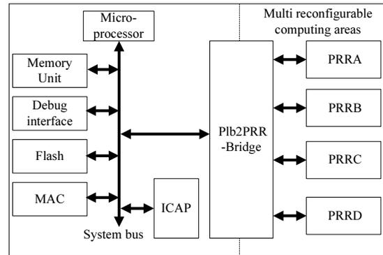
Fig. 2. Reconfigurable computing node function modules
