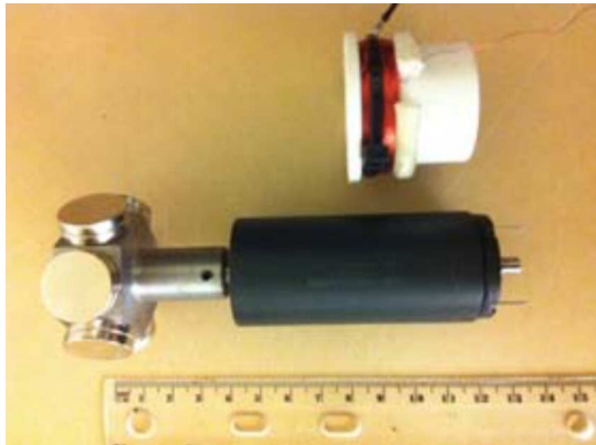
Fig. 3. The picture of the DC motor and the receiving coil used in this paper. The motor is from Faulhaber (Model: 3272G012CR). The coil is hand-wound with 600 turns and a diameter of 34 mm. The wire diameter is 0.025 mm.
