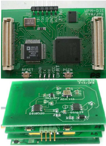
Fig. 1. On the top part, the Cookie processing layer (uC on the left and the FPGA on the right) and on the bottom, a complete Cookie node.
