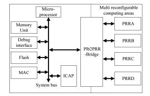
Fig. 2. Reconfigurable computing node function modules
