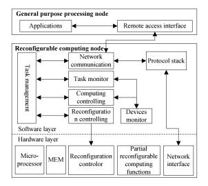
Fig. 1. System function module architecture
