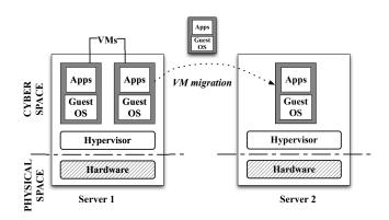
Figure 1. Virtualization software, the hypervisor, is used to partition the physical resources of servers for virtual machines (VMs), allowing the usage of a data center as a utility. Virtualization allows separation of the physical components of the servers from the cyber components which are the VMs and which can be migrated among the physical servers.
