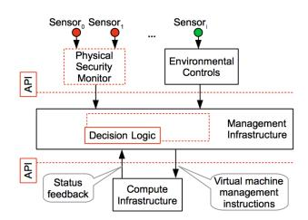
Figure 3. The components of our proposed system. The three new key components are shown in dashed lines: Physical Security Monitors, API and Decision Logic.
