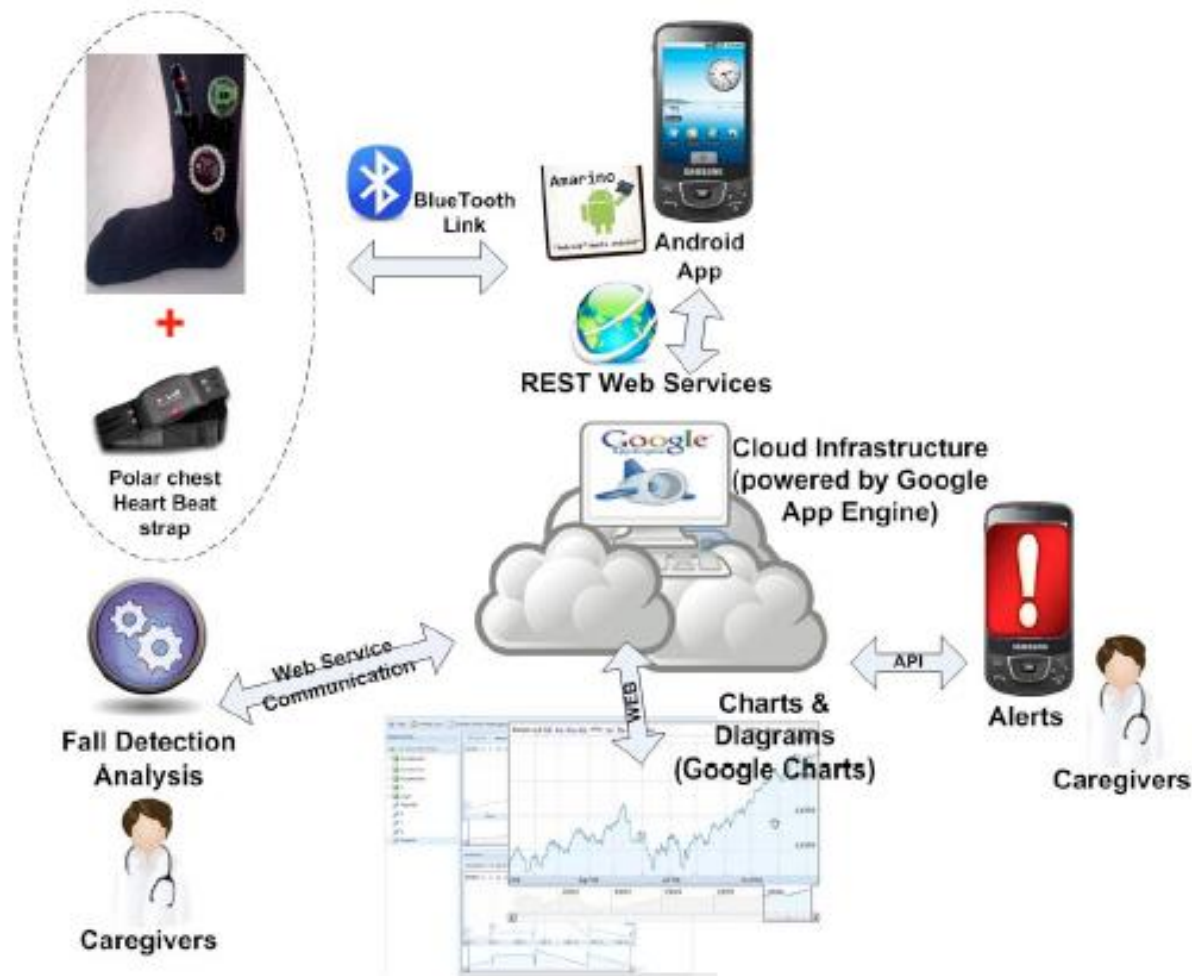
Figure 2. Illustration of the architecture, main components and interaction with users.
