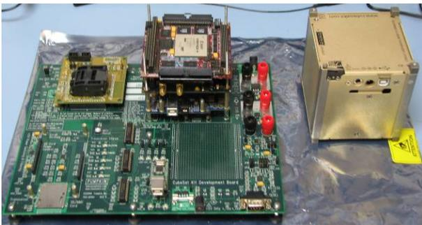
Figure 2. CubeSat Platform with Flight Module, IEEE 802.11 Board and FPGA Board
