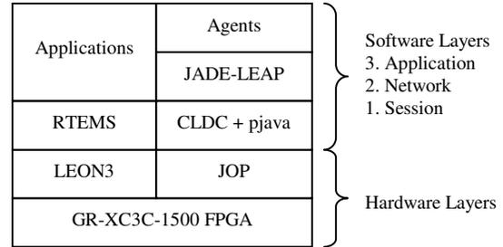
Figure 5. Hardware & Software Layer Design
