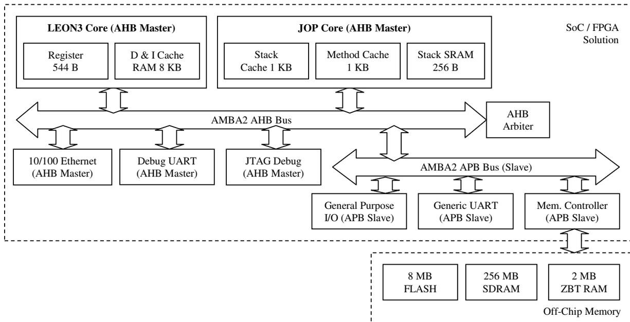
Figure 7. System-on-Chip Block Diagram
