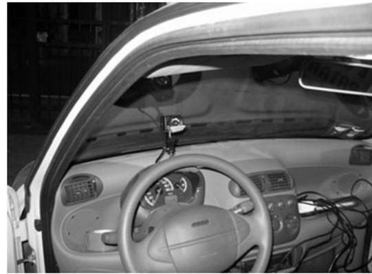
**Fig. 7** The IR CCD camera on the car dashboard
