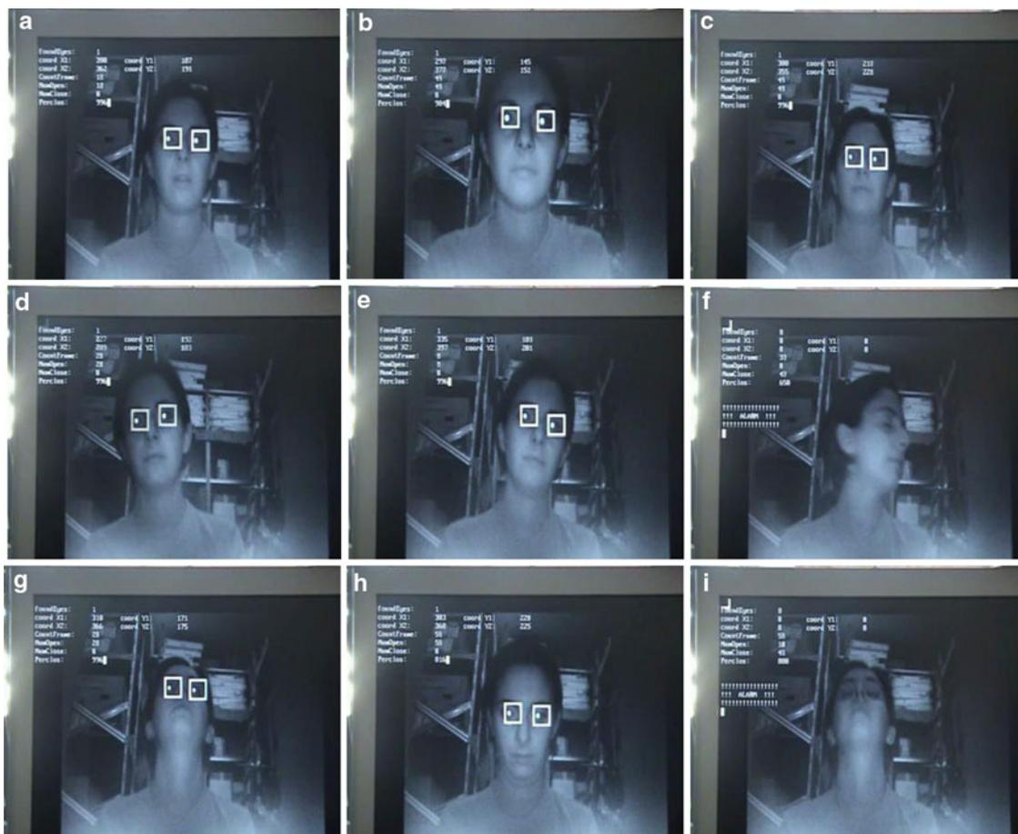
**Fig. 8** System evaluation—Snapshots from video 1 (frames **a**, **b**, and **c**), and video 2 (frames **d**, **e**, **f**, **g**, **h**, and **i**). Tracked driver’s eyes are marked with *white squares*. System performance is not affected by driver–camera relative distance (frames **a**, **b**, and **c**), by driver’s head
