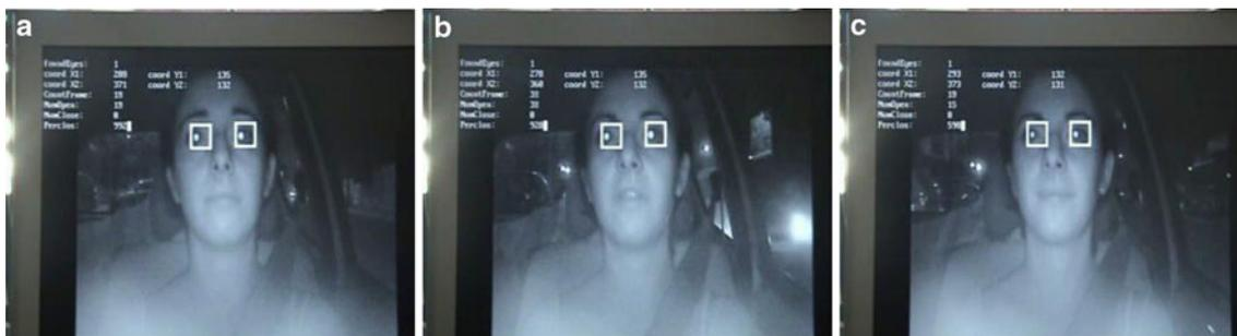
**Fig. 9** System evaluation—Snapshots from video 3 (frames **a**, **b**, and **c**). The environment is very noisy due to the several external light sources (cars, unidentified city lights). Tracked driver’s eyes are marked with *white squares*
