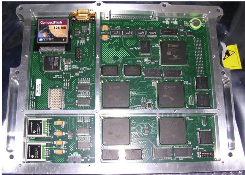
Figure 2. Photograph of the MSP Flight Engineering Model.
