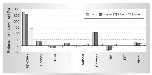
Figure 4. Performance improvement with the clustered vector organization. The FFT benchmark shows a 0 percent performance degradation.
