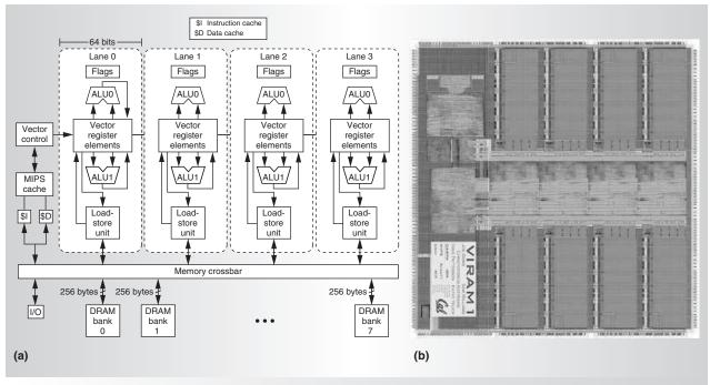
Figure 1. VIRAM prototype processor: block diagram (a), die photo (b).
