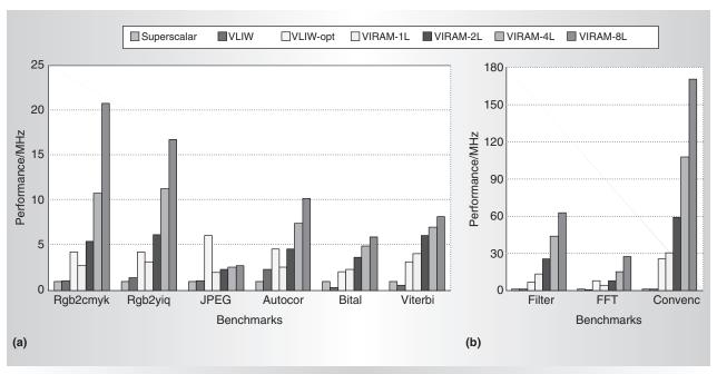
Figure 2. Performance-per-MHz comparison, normalized to the performance of the MPC7455 superscalar processor. Note the change of scale between the benchmarks in (a) and those in (b).
