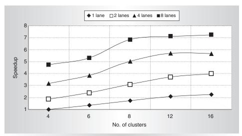
Figure 5. Average speedup for the EEMBC benchmarks with scaling of the clustered vector processor.
