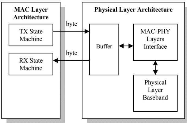
**Figure 7. MAC layer 's Interface with Physical Layer**
