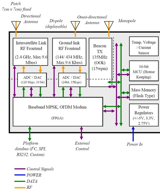
**Figure 10. Intersatellite Communications Module Functional Block Diagram**
