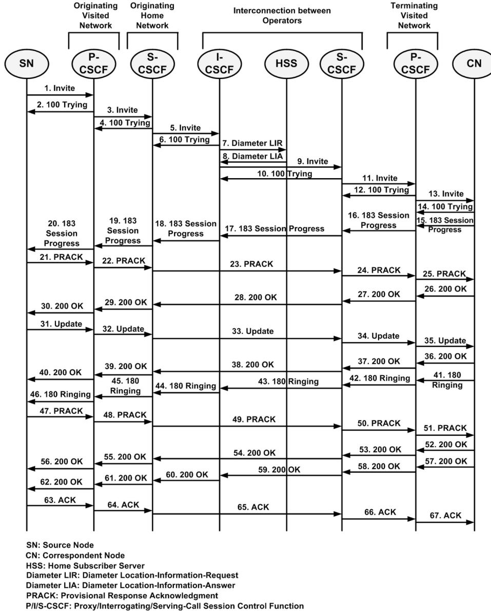
Fig. 5. The IMS session setup process (adapted from [30], [31]).
