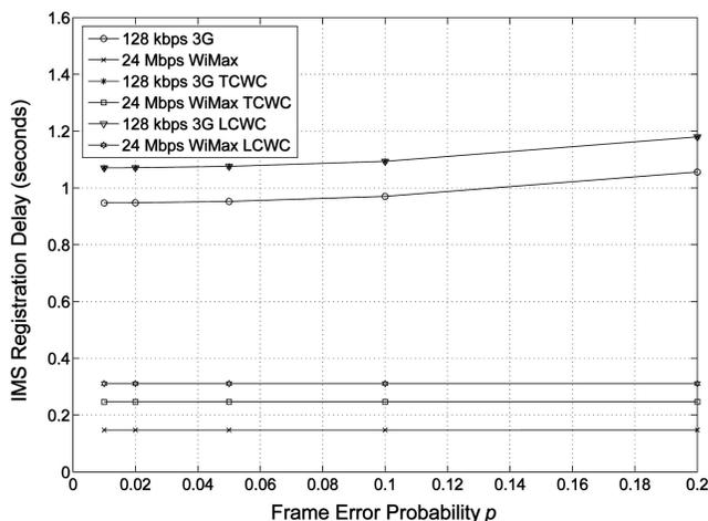
Fig. 10. The effect of varying frame error probability  $p$  on the IMS registration signaling delay for 128 kbps 3G and 24 Mbps WiMax networks with a fixed signaling arrival rate  $\lambda$ .
