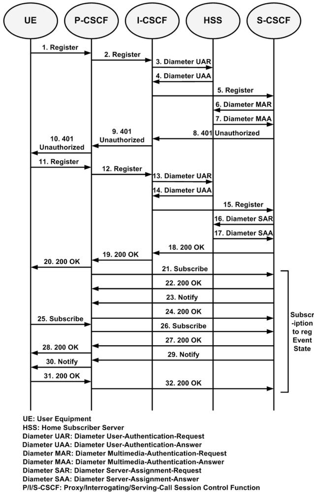
Fig. 4. The IMS registration process (adapted from [30], [31]).
