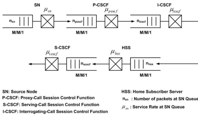
Fig. 6. Queuing network for IMS registration process.
