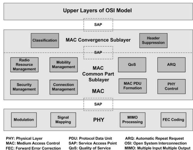
Fig. 1. WiMax protocol stack (adapted from [24]).
