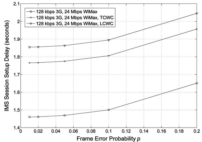
Fig. 11. The effect of varying frame error probability  $p$  on the IMS session setup delay when the SN is in a 128 kbps 3G network and the CN is in a 24 Mbps WiMax network for a fixed signaling arrival rate  $\lambda$ .
